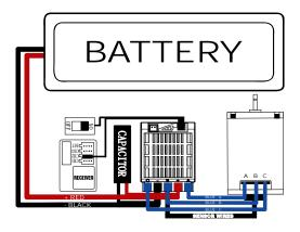
To avoid radio glitches, arrange the placement of the ESC such that the power wires and the receiver antenna wires do not cross over each other.
